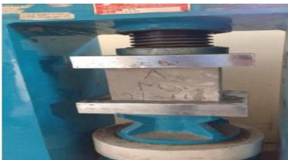
Fig. 1. Setup of Compression Strength Testing Machine.
